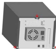
Power off and remove 3 screws in back
