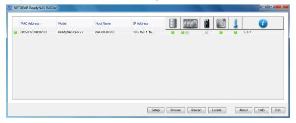
The default IP configuration is set to DHCP, which is how home routers assign IP addresses by default.
