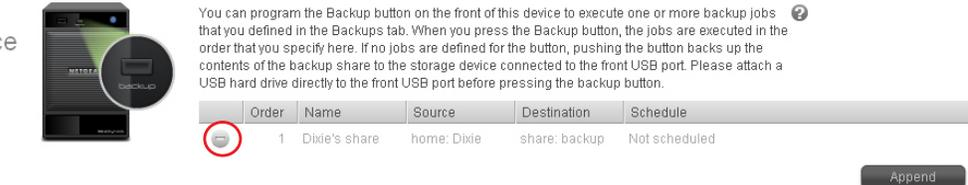
You can program the Backup button on the front of this device to execute one or more backup jobs that you defined in the Backups tab. When you press the Backup button, the jobs are executed in the order that you specify here. If no jobs are defined for the button, pushing the button backs up the contents of the backup share to the storage device connected to the front USB port. Please attach a USB hard drive directly to the front USB port before pressing the backup button.
