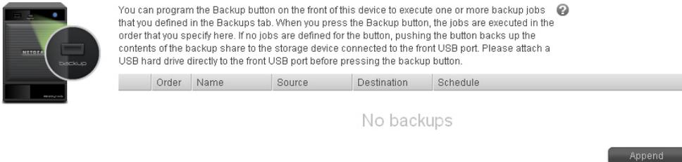
You can program the Backup button on the front of this device to execute one or more backup jobs that you defined in the Backups tab. When you press the Backup button, the jobs are executed in the order that you specify here. If no jobs are defined for the button, pushing the button backs up the contents of the backup share to the storage device connected to the front USB port. Please attach a USB hard drive directly to the front USB port before pressing the backup button.
